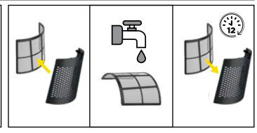
3. OPTIONAL: If debris is stuck between the mesh filter and the Dust Defence panel, the filter can be removed by gently pulling it out of the tabs on the panel. Rinse the filter and the panel with room-temperature tap water. Allow both the filter and the panel to air-dry for 12 hours before reinstalling. DO NOT use the fan when the mesh filter is wet.
