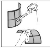
Use a vacuum cleaner on low speed with a soft brush attachment OR a cloth/towel to remove debris from the Dust Defence panel and the internal mesh screen.
