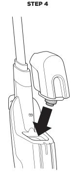
**4** To replace the water tank, align it so the cap faces down. Place the cap into the hole in the Steam Mop body and slide tank down until it clicks securely into place.
